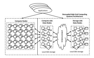
Decoupled HPC System Architecture
