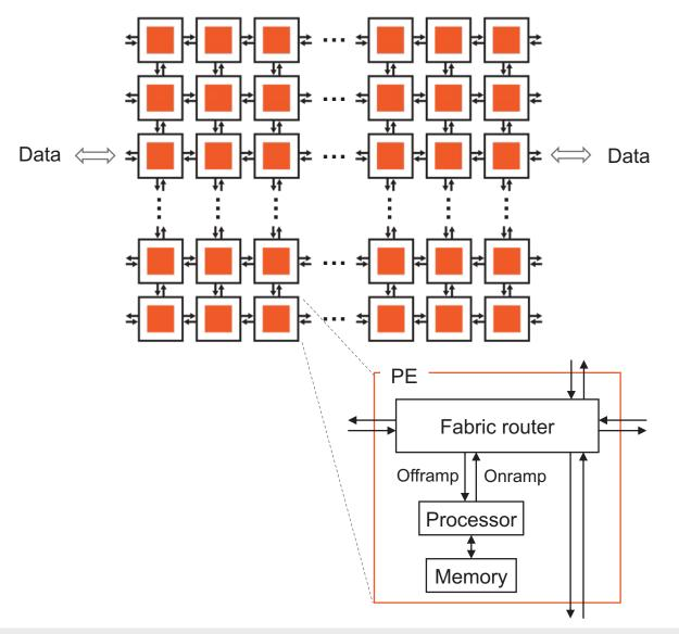
The CS-2 appears as a logical 2D array of individually programmable Processing Elements
